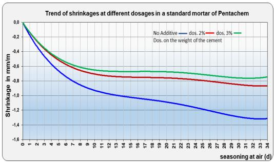
The values have been recorded on mortar composed by 42.5 II/A-LL cement, normal sable, and water
